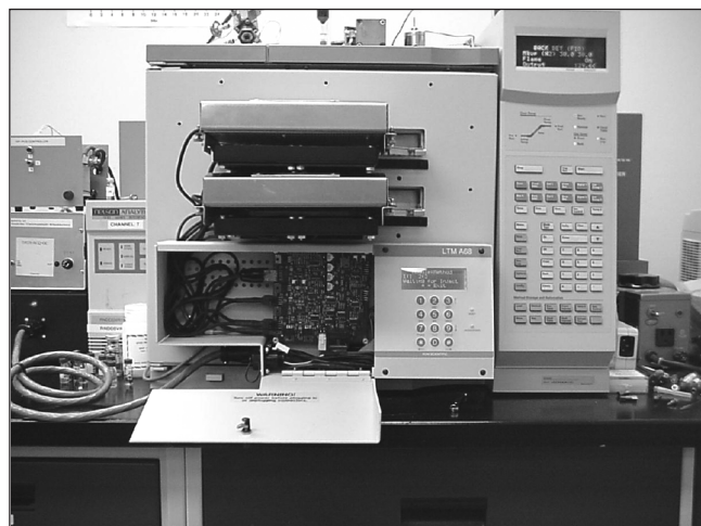
Figure 1. Picture of an Agilent HP-6890A used for stacked injection with LTMGC. Note the two modules mounted on the oven door. Module 1, 2-m \times 0.53-mm i.d., CP-Lowox connected in series to Module 2, 25-m \times 0.32-mm i.d., 1.2 \mu m CP-52CB.
